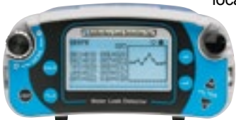
The "Saved" data file showing 10 leak sound levels and graphical display. Leak is at the peak sound level in the center.
