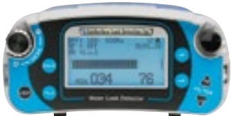
LD-18 Amplifier showing filter settings, bar graph and numeric display of sound loudness, and minimum sound level detected
